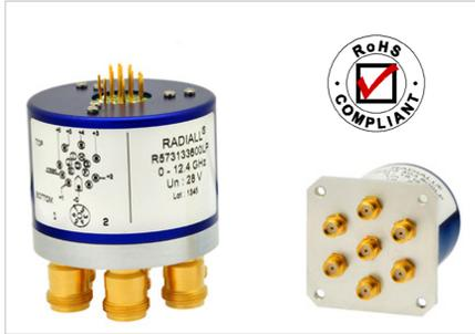
To meet growing market demands created by the deployment of 4G/LTE networks, Radiall has introduced a new range of Low PIM switches. RAMSES SPnT Low PIM switches are perfectly suited for RF test systems and test benches requiring excellent passive intermodulation performance up to 18 GHz, with a guarantee PIM performance of -160 dBc @ +43 dBm over a life span of 2 million switching cycles.
