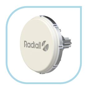
Radiall's V-Band mmWave antenna is perfectly suited for integration in new telecom systems, where small form factor and high gain are critical. This new solution provides 32 dBi bore sight gain from 57 to 66 GHz coinciding with the normal axis of the antenna. This feature helps to facilitate quick and easy alignment between radio units (optical technology or not), which is mandatory for applications such as small cells, backhaul/fronthaul links and WiGig.
