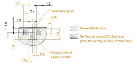
Vias and transmission line inside PCB are not represented. The impedance of the transmission line should be 50 ohms
