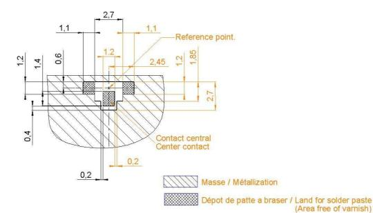
Vias and transmission line inside PCB are not represented. The impedance of the transmission line should be 50 ohms
