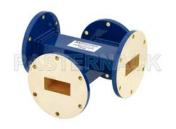
WR-137 50 dB Waveguide Crossguide Coupler, UG-344/U Round Cover Flange, 5.85 GHz to 8.2 GHz
