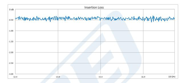
WR-62 Seamless Flexible Waveguide 24 Inch, UG-1665/U Square Cover Flange Operating From 12.4 GHz to 18 GHz from Pasternack Enterprises has same day shipment for domestic and International orders. Our RF, microwave and millimeter wave products maintain a 99.4% availability and are part of the broadest selection in the industry.
