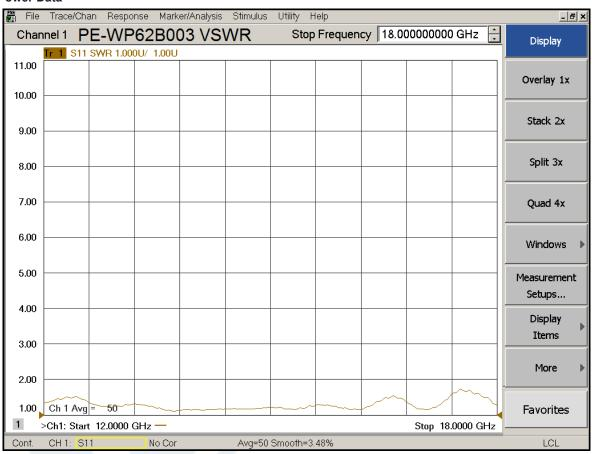
Click the following link (or enter part number in "SEARCH" on website) to obtain additional part information including price, inventory and certifications: WR-62 Instrumentation Grade Waveguide E-Bend with UG-419/U Flange Operating from 12.4 GHz to 18 GHz PE-W62B003
