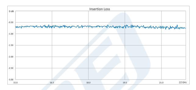
WR-51 Seamless Flexible Waveguide 36 Inch, Square Cover Flange Operating From 15 GHz to 22 GHz from Pasternack Enterprises has same day shipment for domestic and International orders. Our RF, microwave and millimeter wave products maintain a 99.4% availability and are part of the broadest selection in the industry.
