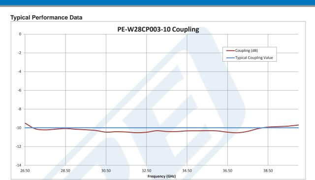
Click the following link (or enter part number in "SEARCH" on website) to obtain additional part information including price, inventory and certifications: WR-28 10 dB Directional Waveguide Coupler With UG-599/U Flange and E-Plane Coupled Port From 26.5 GHz to 40 GHz Ka Band PE-W28CP003-10
