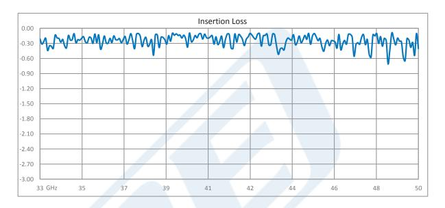
WR-22 Seamless Flexible Waveguide 24 Inch, UG-383/U Round Cover Flange Operating From 33 GHz to 50 GHz from Pasternack Enterprises has same day shipment for domestic and International orders. Our RF, microwave and millimeter wave products maintain a 99.4% availability and are part of the broadest selection in the industry.
