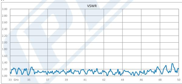
Click the following link (or enter part number in "SEARCH" on website) to obtain additional part information including price, inventory and certifications: WR-22 Seamless Flexible Waveguide 24 Inch, UG-383/U Round Cover Flange Operating From 33 GHz to 50 GHz PE-W22SF005-24
