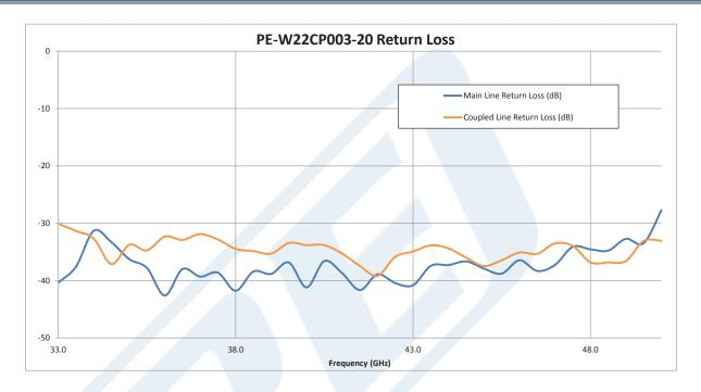
WR-22 20 dB Directional Waveguide Coupler With UG-383/U Flange and E-Plane Coupled Port From 33 GHz to 50 GHz Q Band from Pasternack Enterprises has same day shipment for domestic and International orders. Our RF, microwave and millimeter wave products maintain a 99% availability and are part of the broadest selection in the industry.
