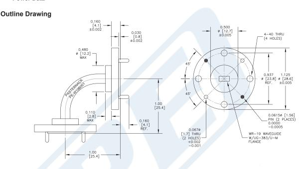
WR-19 Instrumentation Grade Waveguide E-Bend with UG383/U-Mod Flange Operating from 40 GHz to 60 GHz from Pasternack Enterprises has same day shipment for domestic and International orders. Our RF, microwave and millimeter wave products maintain a 99% availability and are part of the broadest selection in the industry.
