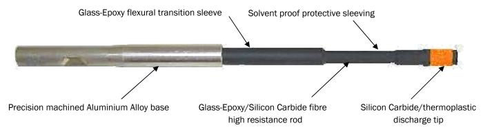
Combining Silicon Carbide and Glass-Epoxy materials, the 21-90-35 is an immensely strong, high performance Static Discharger intended for use on military aircraft operating at speeds in excess of Mach 2.
