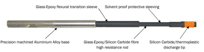
Combining Silicon Carbide and Glass-Epoxy materials, the 21-90-33 is an immensely strong, high performance Static Discharger intended for use on military aircraft operating at speeds in excess of Mach 2.
