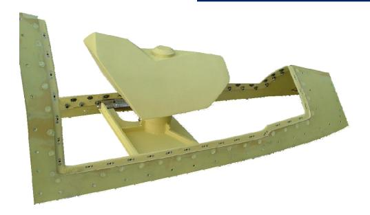
The 21-66-16 is a Special-to-Type multifunction antenna designed to fit conformally into a supersonic military aircraft. The concept is to provide a dielectric "window" (P/N 21-60-16) in the upper surface of the aircraft, through which a combined Line-of-Sight "LOS" and UHF Satcom antenna radiate, using the aircraft structure as a ground plane and reflective surface.
