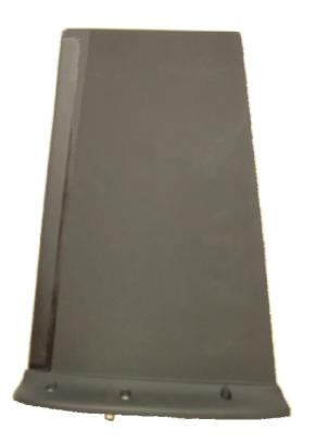
The 21-50-91/92/93 are vertically polarized, omni-directional antennas, compatible with all popular airborne radios operating within the 30 to 400 MHz frequency range. These antennas can handle 100 Watts of power and require no external tuning.
