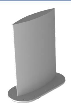
The 21-50-115 is a low profile blade antenna providing excellent VHF and UHF performance in a small passive design over the entire frequency band of 30-512 MHz. Radiating element design is optimized to provide excellent omni-directivity in azimuth over the full band in a low drag, elliptical shaped structure.
