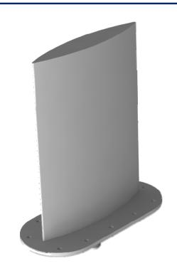
The 21-50-114 is a low profile blade antenna providing excellent UHF and L-Band performance while also providing frequency coverage in the 30-88 and 108-174 MHz bands. Radiating element design is optimized to provide excellent gain and omni-directivity in azimuth over the full 225-512 MHz and 960-1220 bands while VHF provides moderate performance only due to the antenna's very low height.
