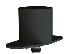
The 21-40-33 is a multifunction airborne data link antenna providing vertical polarisation for 1625 to 5850 MHz with radiation similar to a stub and right hand circular polarization from 14.4 to 15.4 GHz with an essentially downward looking (when mounted underneath the air vehicle) radiation pattern.
