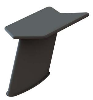
The 21-30-76-1 is a rugged UHF Satcom antenna designed for airborne, ground and shipborne applications. A high strength aerodynamic vertical shell supports a "Bat-Wing" shape horizontal element containing a pair of cross dipoles, connected to provide right hand circularly polarized UHF Satcom coverage including MUOS frequencies.
