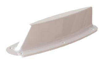
The 21-20-79 is a lightweight Marker Beacon Antenna suitable for Instrument Landing Systems (ILS) installations on helicopters and subsonic aircraft. Its rugged design uses a printed circuit radiating element enclosed within a lightweight glass reinforced composite shell which in turn is bonded into a machined aluminum alloy base plate. This method of construction avoids base delamination problems associated with some other manufacturers designs.
