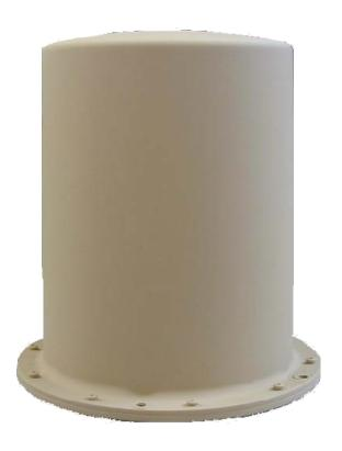
Designed to provide optimum performance in a low height, type 20-50-60 is a discone type wide band antenna build into a rugged cylindrical Radome capable of withstanding typical military vehicle operations. This antenna is one of CAL's multiband designs particularly suited to special mission and on-the-move operations. This version has a flat base of 13 inches diameter for surface mounting on a vehicle with the connector projecting thru the skin into the vehicle.
