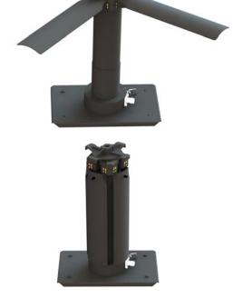
The 20-30-10 series are combined Hi-Lo angle UHF Satcom Antenna designed for installation on a vehicle roof, shelter or housing via either a fixed or magnetic base. The 21-30-10 series has 4 spring loaded elements which can be easily and immediately deployed.
